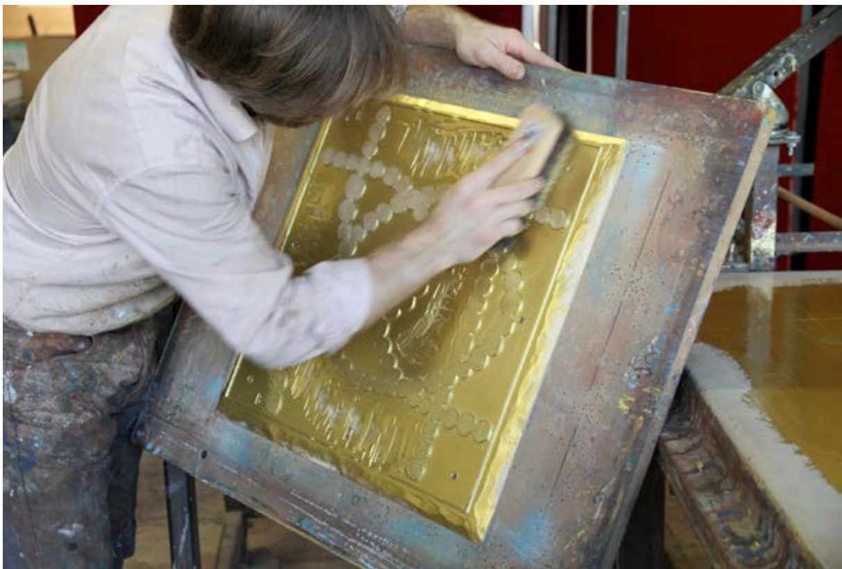
Work session on the embossed plates for the handmade wallpaper, Atelier d'Offard, 2014.
